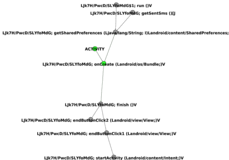
Figure 6.12.: The subgraph of the call graph generated by Androguard that is rooted at the entry callback method onCreate . Note that only two internal methods, finish and getSharedPreferences , that are directly invoked as shown in Figure 6.5 are detected. The other methods shown here also invoke (one of) these two methods, but are not invoked from onCreate .
